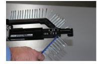
To remove the strip, pull it through the auto-feed end assembly.
