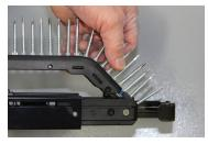
Feed the strip into the slide body until the 2nd empty slot is aligned with the bit. The tool will feed the first screw when depressed against the work surface.
