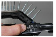
The screw gun is preset from the factory for a 2" screw. Confirm that it is still set at the 2" mark.
