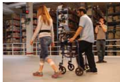
A researcher from The Ohio State University takes tibial shock readings on a ResinDek® mezzanine
